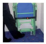
2. Remove the chair from the wall and place on the ground. Engage the footbrakes by pressing down on the foot pedals on BOTH brakes shown in the picture.
