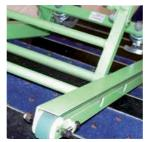
11. Keeping the tracks firmly in contact with the stairs, ensure a firm grip, apply downwards pressure on the handle and allow the chair to operate downwards.
