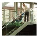
11. Manoeuvre the chair forward onto the top two steps, make sure the tracks stay in full contact with the stairs.
