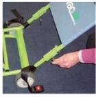
3. Unfold the handle and insert the safety pins on each side to secure.
