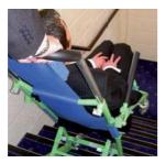
10. Hands are now placed on top of the handle, tilt the chair back and manoeuvre over the edge of the stairs.
