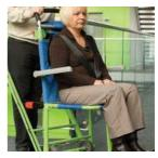
6. Transfer the client into the chair, as per the personal emergency evacuation plan (peep), fasten the support harness and bring over the arms.
