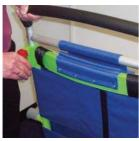
15. Undo the red spring clips on the handle and gently lower, close the red spring clips and lift the handle until it locks into place. Pass support harness through and over the handle.
