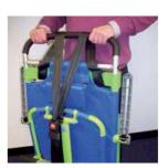
17. Pass the lower part of the support harness through the foot rest and connect to upper harness. Place chair back into storage location and replace protective cover.
