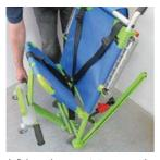
4. Release the support strap, open the chair from the side to a seating position, using the black handle and then ensure that it is locked into place, by pushing down on the bar with the two red locks.
