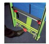
14. Ensure the brake mechanism is locked.
