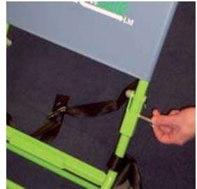
3. Remove the safety pins on each side of the handle and fold the handle down.
